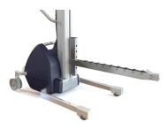
Roller boom Equipped with rollers for effortless loading and unloading of reels. Safety pin for safe transportation.
