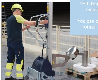
TAWI Lifting Trolleys are easy to maneuver and push forward making it almost effortless to transport goods to the intended location. You can pick up goods from a vertical or horizontal position, rotate, transport, turn and release with minimum effort.
